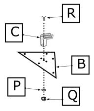
THE REMAINING 4 RIB BRACKETS-C, ARE ATTACHED TO POST BRACKETS-B, WITH M5 BOLTS-R, WASHERS-P AND NUTS-Q.
