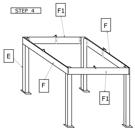
ONCE TWO END SECTIONS ARE ASSEMBLED, STAND THEM UP AND BOLT THE OTHER TWO CROSSRAILS-**F1** INTO POSITION.
